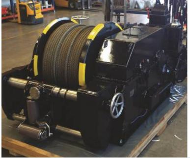
Towing winches come in different configurations like single and double drums, waterfall or in-line configuration, with rated pull up to 150 tons. Manual and remote clutch operation is standard with also automatic emergency functions, constant tensioning mode and static brake slippage.
