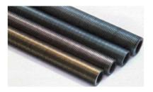
Low Fin (Integral) tubing is a type of extruded tubing that consists of small low fins. The low fin tube is very similar to the extruded "high fin" types but these tubes have the same diameter as the base tube. Low Fin Enhanced tubes can be used in standard shell and tube baffles and t ube sheets. The primary advantage for the low fin tube is providing surface enhancement and better heat transfer over smooth tubing.
