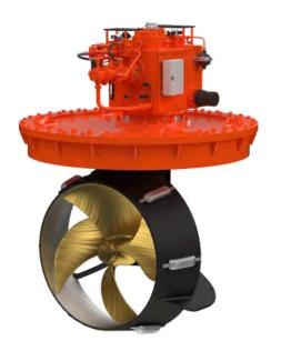
Veth Propulsion's L-Drive/Z-Drive azimuth thrusters are designed for ultimate maneuverability, efficiency, and reliability. The 360-degree rotation around the vertical axis allows full thrust in any direction, making them ideal for various marine applications, from inland vessels to offshore operations, mega yachts and more.
