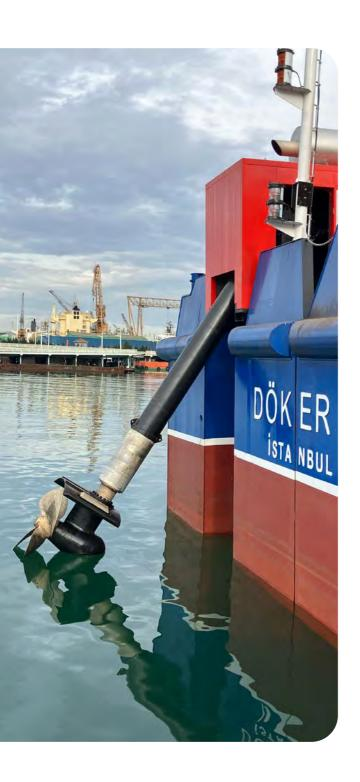
If your vessel is not equipped with an engine room, then a Deck-Mounted Thruster may provide an interesting solution.
