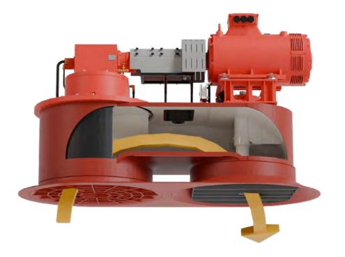
Water intake occurs through the propeller opening beneath the vessel, guided outward through a hydrodynamically streamlined housing. This grid, directly controllable across 360 degrees, enhances maneuverability and control. Compact in design, the gearbox minimizes exterior pipework, while critical
