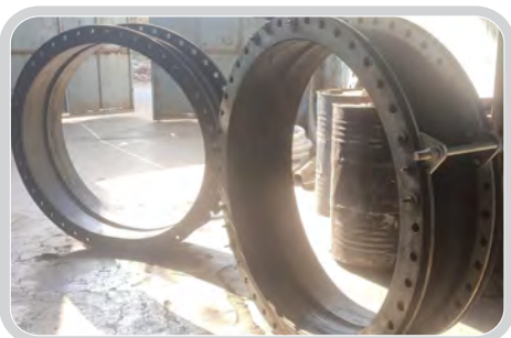
RUBBER EXPANSION JOINT SPLIT FLANGE
