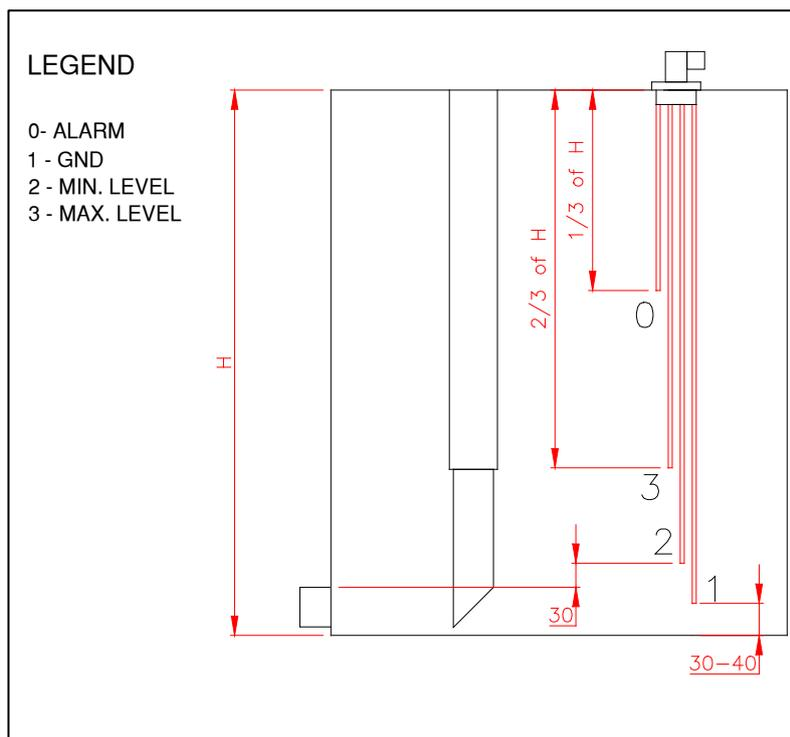
**Fig. 8.6.1.1-2 - Collecting tank and 4-rods level sensor**
