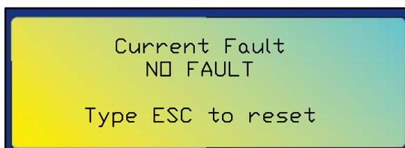
Press again the STOP/ESC key to return to the system main page. Then, restart the plant by pressing the START/ENTER key, the system will begin to run from the filling step.
