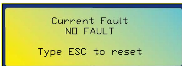
Press again the STOP/ESC key to return to the system main page. Then, restart the plant by pressing the START/ENTER key, the system will begin to run from the filling step if the liquid level inside the Treatment Tank is below the min level of multilevel sensor; otherwise from the chemical dosing phase.
