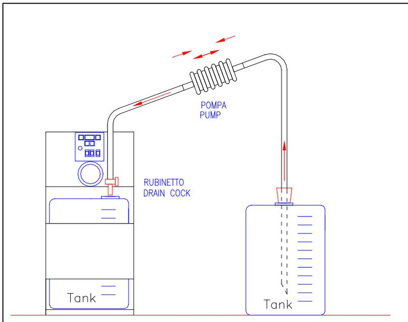
**Fig. 8.6.3.1-1 - Filling the dosing system tank**
