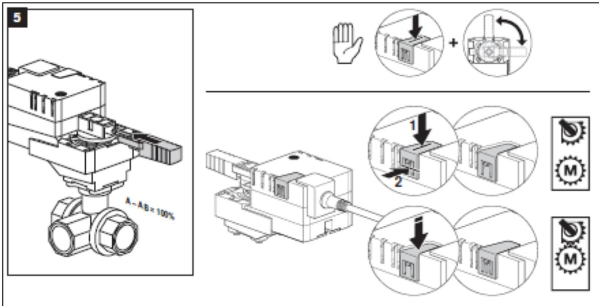
**Fig. 13.1.1-1** –Manual opening activation for motorized valves V1 & V2 (ECOMar 20 S-32 S -45 S-70 S-145 S)
