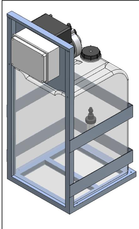
**Fig 8.8.2 – H<sub>2</sub>O<sub>2</sub> dosing system for 2 Tanks Control configuration**
