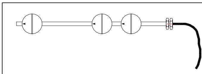
**Fig. 12.3.2-1 – Multi-level sensor installed on the Treatment Tank for ECOMar 20 S- 32 S - 45 S - 70 S – 145 S**
