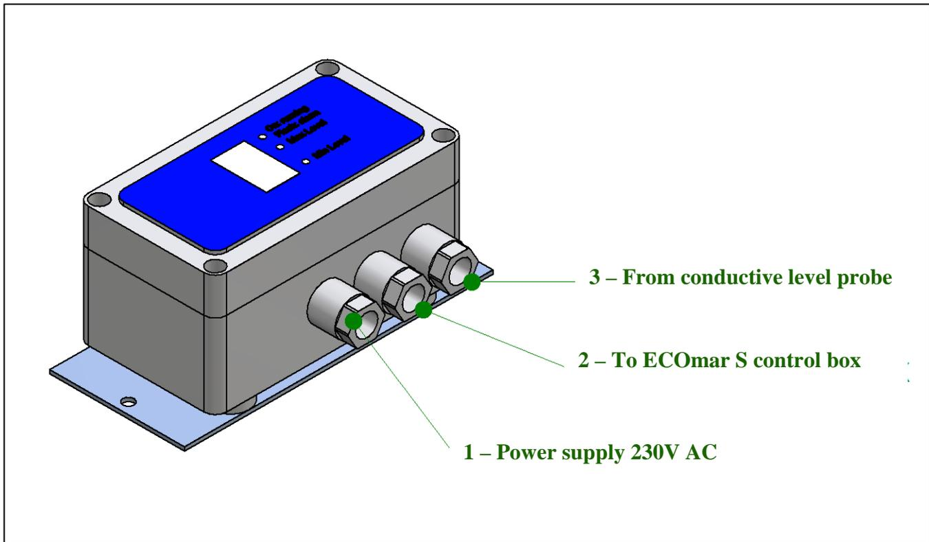
**Fig 8.8.3 - Electrical connection of the control box for level probe**
