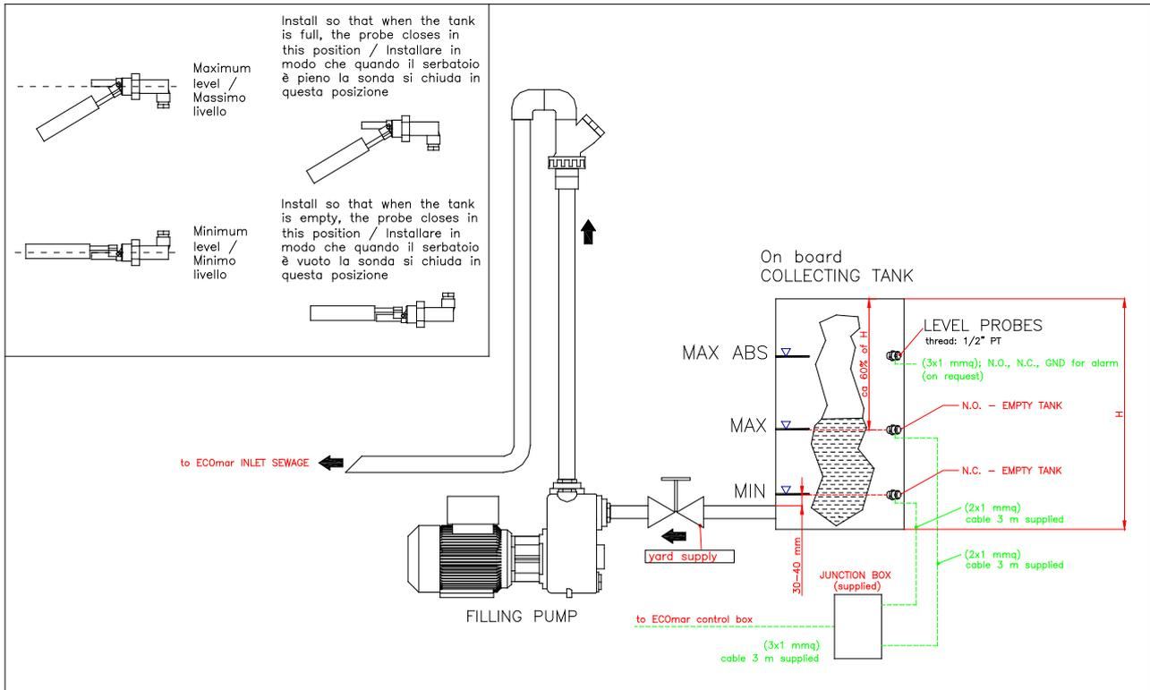
**Fig. 8.6.1.1-3 - Collecting tank and lateral mounting level probes**
