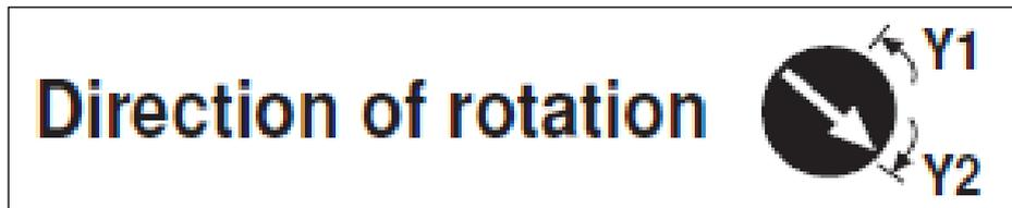
**Fig. 10.1-1 – Indicator for the sense of rotation\* of the motorized valves (V1) & (V2)**
