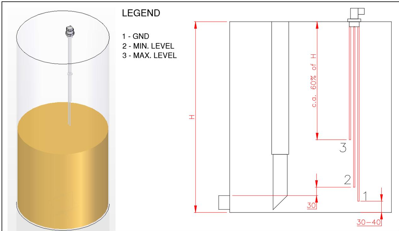
**Fig. 8.6.1.1-1 - Collecting tank and 3-rods level sensor**
