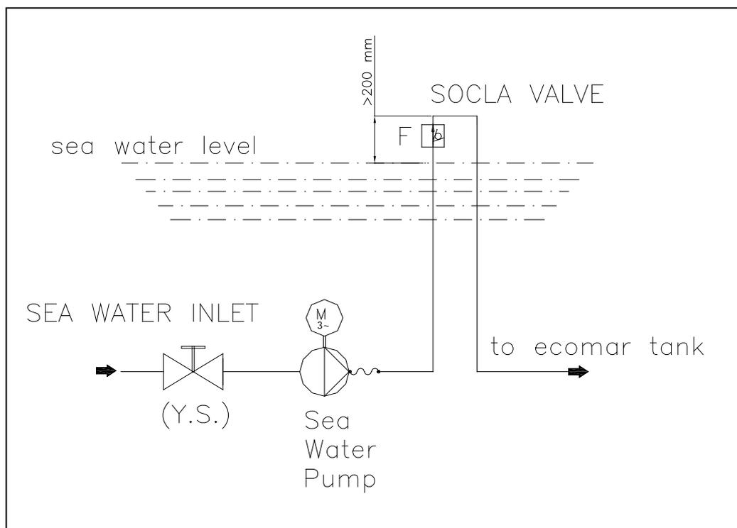
**Fig. 8.6.2 - Connection scheme for Sea Water anti-siphon valve set**
