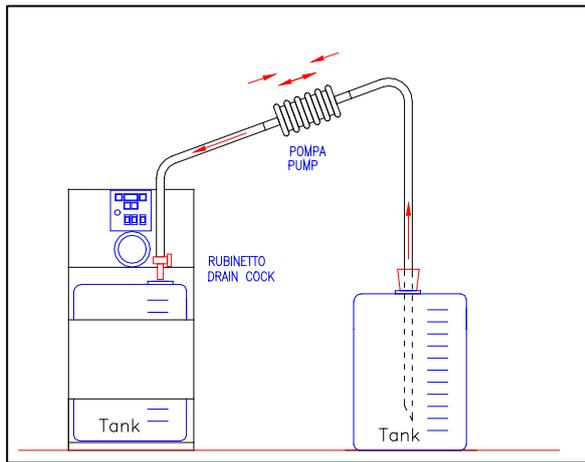
**Fig. 8.6.4.1-1** - Filling the dosing system tank
