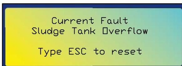
Check that the sludge tank is empty; if it is not, empty it according to IMO/MARPOL regulation, otherwise check the correct functioning of the level probe (your supply) installed on the sludge tank.
