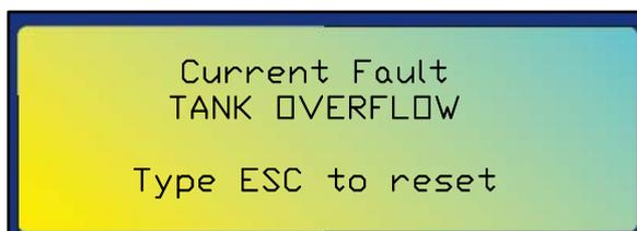
Check the multilevel sensor (ball type) installed on Treatment Tank for any blockages or malfunctioning. Verify that the liquid inside the Treatment Tank is above the Absolute Max level, and empty the treatment tank (refer to the **SPECIAL PROCEDURES** section), resending the liquid back to the collecting tank or discharging it according to IMO/MARPOL regulation. Check that all pumps are working correctly.
