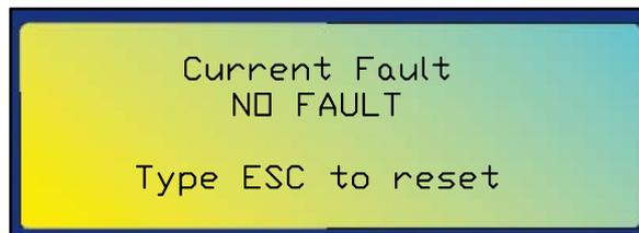
Press again the STOP/ESC key to return to system the main page. Then, restart the plant by pressing the START/ENTER key, the system will begin to run from the filling step if the liquid level inside the Treatment Tank is below the min level of multilevel sensor; otherwise from the chemical dosing phase.
