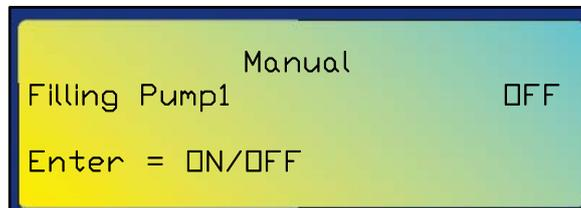
This operation mode allows to manually activate the devices connected to the system. This is useful to check the devices correct functioning when searching for failures, to perform the unit commissioning, plant first start-up or some maintenance operations.
