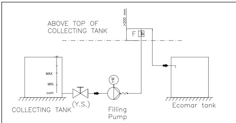
**Fig. 8.6.1.2-1 - Connection scheme for filling anti-siphon valve set**
