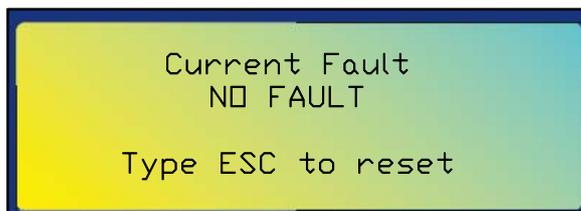
Press again the STOP/ESC key to return to the system main page. Then, restart the plant by pressing the START/ENTER key, the system will begin to run from the chemical dosing phase.
