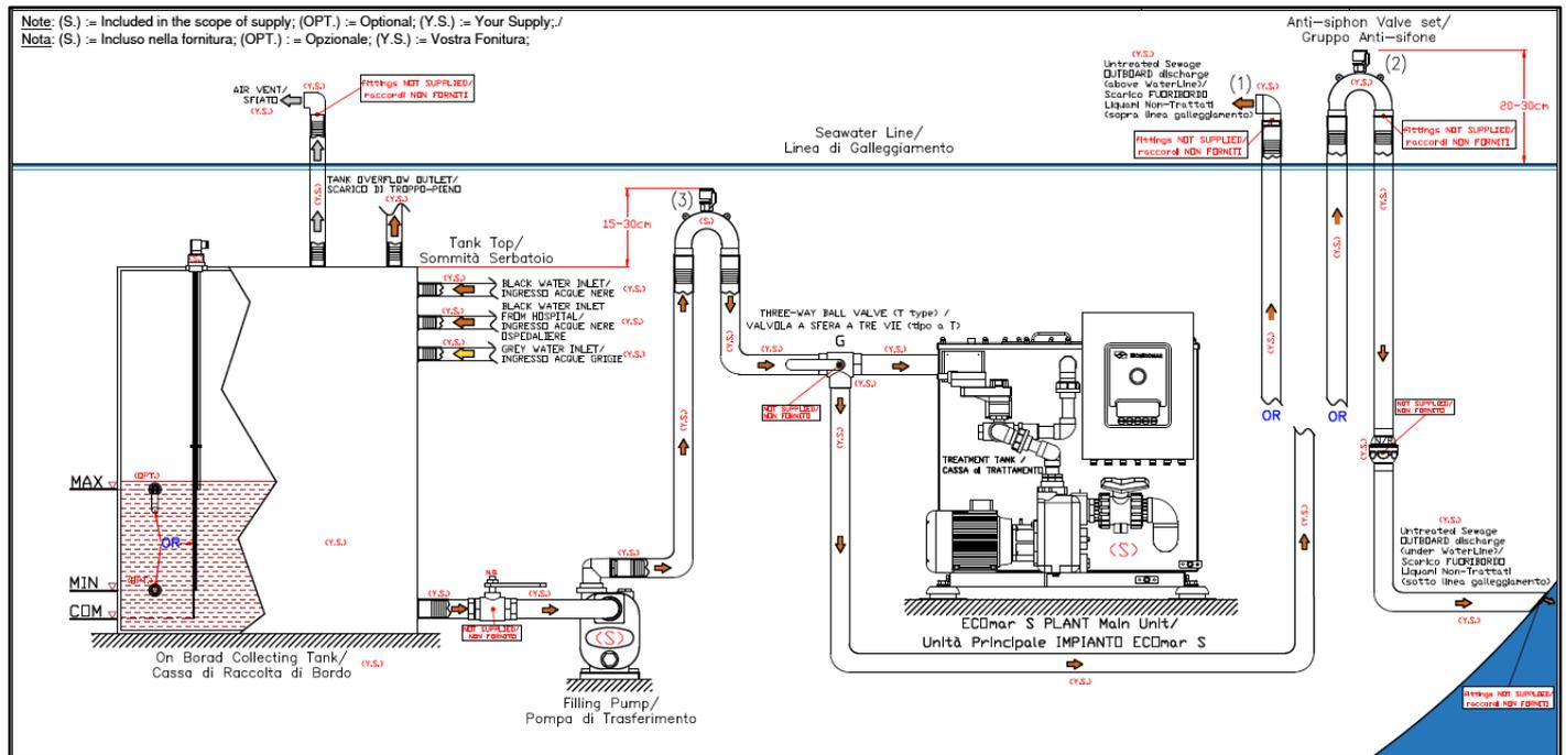
**Fig. 12.1** – Untreated Sewage outboard discharge flow diagram
