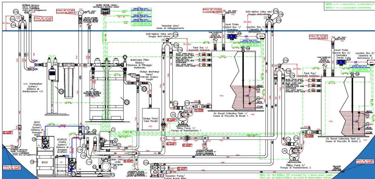
**Fig. 6-2 - Functional installation scheme – 2 Tanks Control - (see also annexed drawing)**
