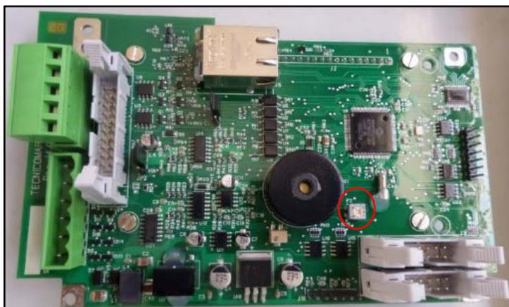
**Fig. 14.3.3 (Trimmer P2 on PRO14 P.C.B. rear side)**
