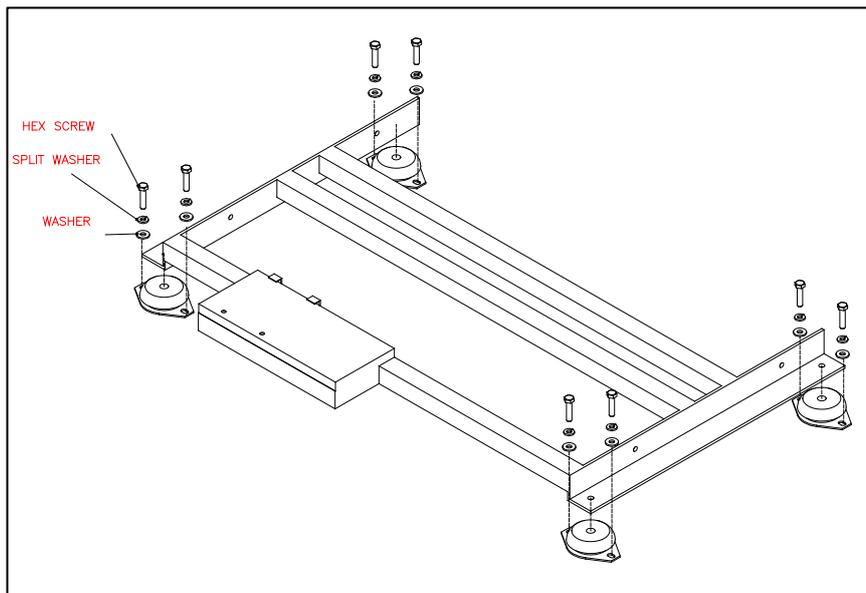
**Fig. 8.3 - Scheme for skid fixing indications**
