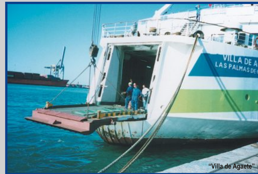
Modification of the stern ramp to connect to link span
