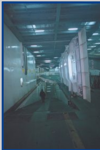
Two-sections pivoting cover over fixed ramp.
