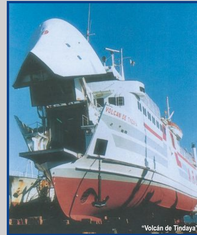
Design and supply of the bow visor operation.-Bow ramp
