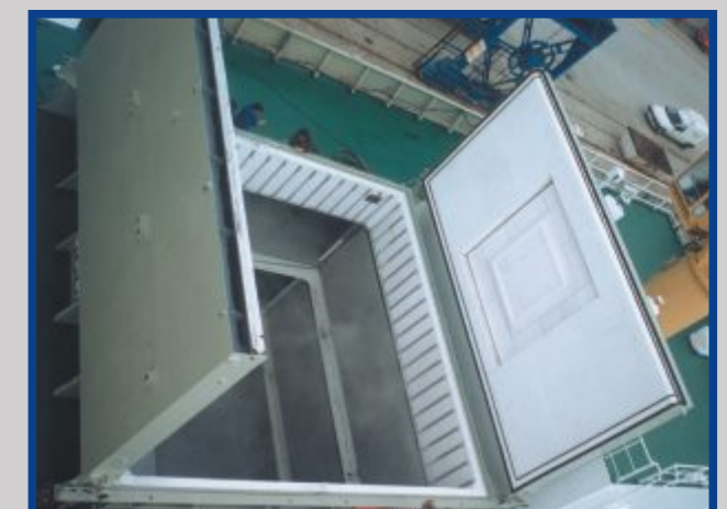
Hydraulic pivoting, insulated, and tweendecks folding
