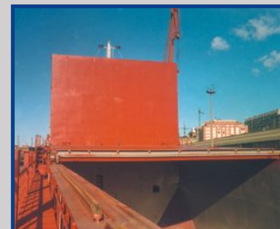
Multifolding on weather deck
