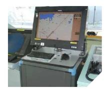
Navmaster ECDIS is an established Electronic Chart Display and Information System, incorporating the input of many navigators and Type-approved to the latest IMO standards.
