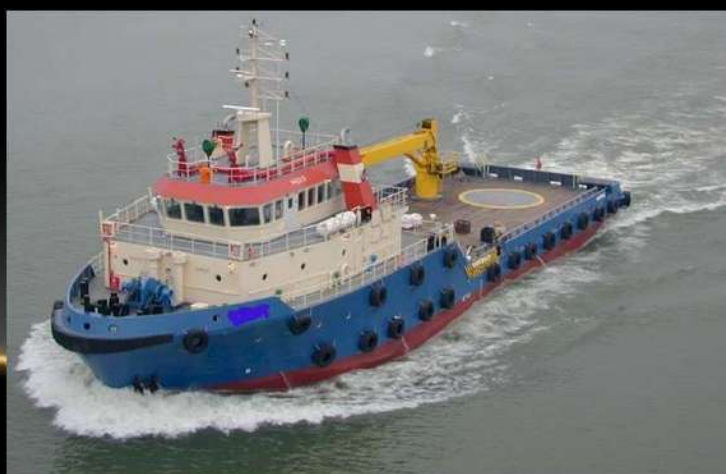
Offshore Supply Vessel – 10 mtr x42 mtr +12 crew built under RINA class
