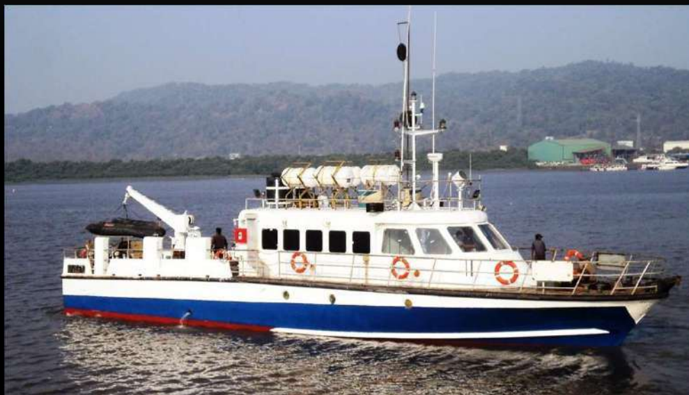
Aquator Crew Boat built by S.P.L under IRS class ,capacity 30 pax + 6 crew. Area of operation - 200 nautical miles from shore , complied under SPS code. ( 1 st time built in India )
