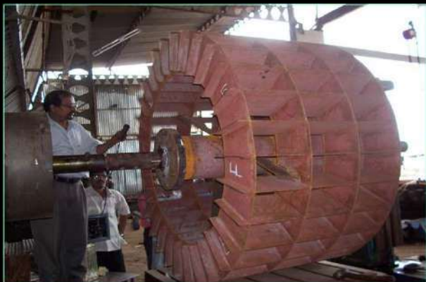
Dynamic Balancing of Blower Impellor
