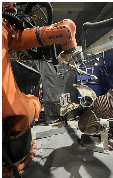
Figure B: Additive Manufacturing of a ship propeller with a diameter of 1050mm
