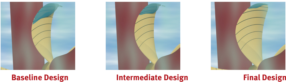
Figure A: Evolution of a low cavitation and underwater noise propeller design
