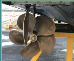
VAR Rudder installed for sea trials
