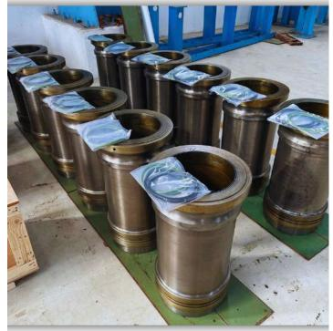
Parts are Stocked after NDTs and Dimensional Inspection
