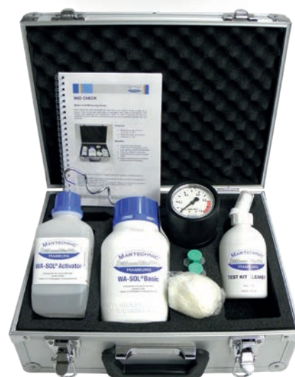
WIO CHECK is delivered as a test kit with necessary reagents and accessories
